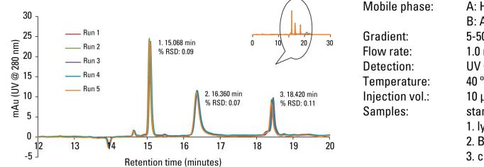
A: H<sub>2</sub>O + 0.05% TFA B: ACN + 0.05% TFA 5-50% B over 20 min 1.0 mL/min UV @ 280 nm 40 °C 10 μL standard protein mixture 1. lysozyme 2. BSA 3. chymotrypsinogen
