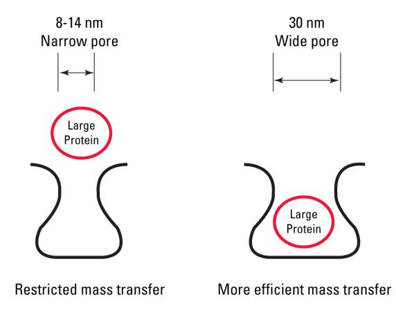
The larger pore size of the TSKgel Protein C4-300 column helps in more efficient mass transfer during chromatographic analysis.
